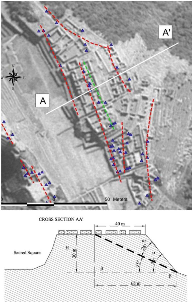
Fig. 2.21 Cross-section of potential unstable planar slide in the NE flank of the citadel adopted for the model. In the upper figure, blue triangles are cracks in structures, dashed red lines are deformation patterns and green line is a tension crack
