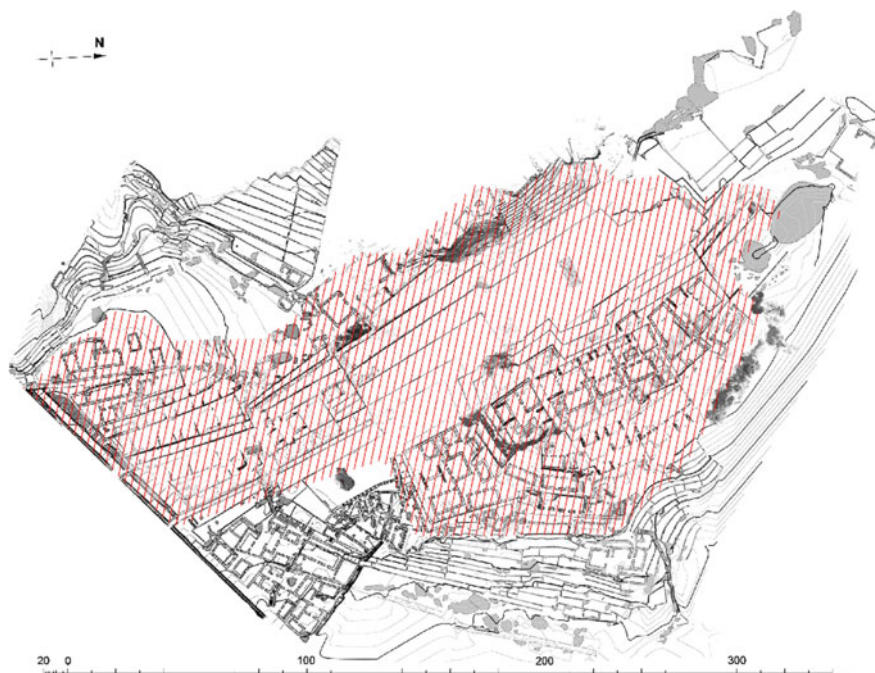
Fig. 9.5 The Llaqta Machupicchu. The red-hatched area indicates the part covered by TLS survey. Drawn by A. Kubicka
