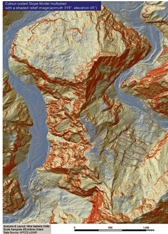
Fig. 8.8 Processed LiDAR data for the central part of the Park (Llaqta de Machupicchu) showing differences in the slope inclination: from flat (blue), through moderate (yellow), to the steepest slopes shown in red. Source Fletcher et al. (2020, p. 386, Fig. 6)
