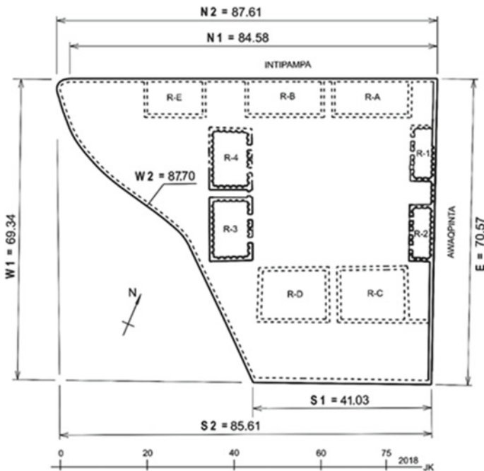
Fig. 9.3 Results of Coricancha EAC and LabScan3D laser survey. Drawing by J. Kościuk
